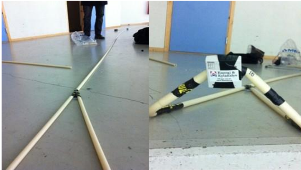
Figure 18 (Left) connected pipe to support the logger and (right) logger used to measure the air temperature in gap between original inner ceiling and low e-ceiling
