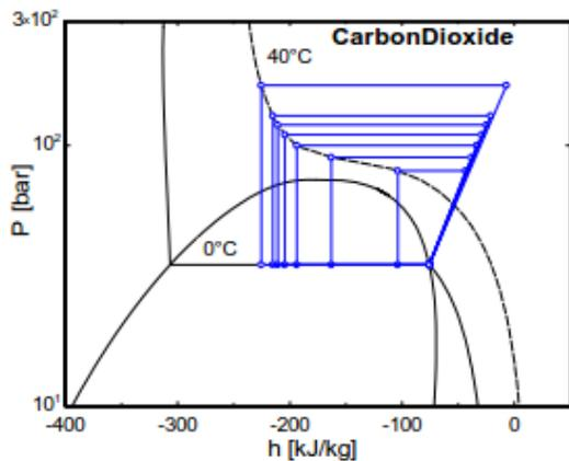
Figure 7 CO<sub>2</sub> transcritical cycles with a 40°C gas cooler exit and different discharge pressures
