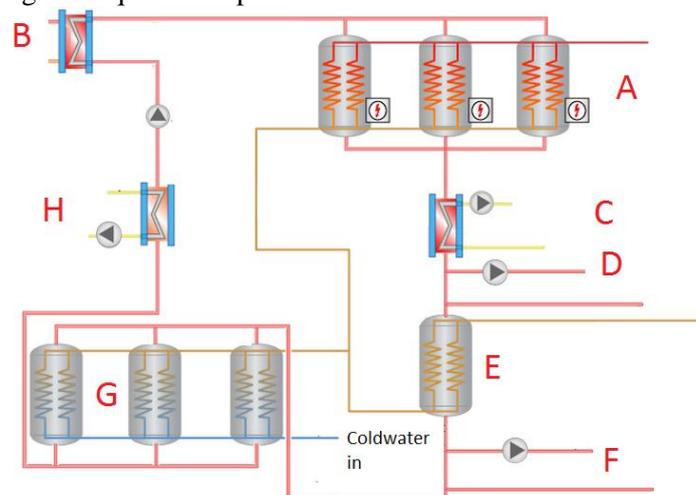
Figure 4 Schematical view of the heat recovery system.
