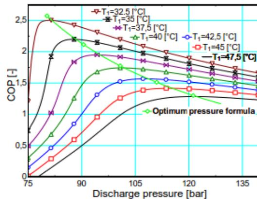
Figure 8 COP<sub>2</sub> of transcritical CO<sub>2</sub> cycle vs discharge pressure for different gas cooler exit temperatures
