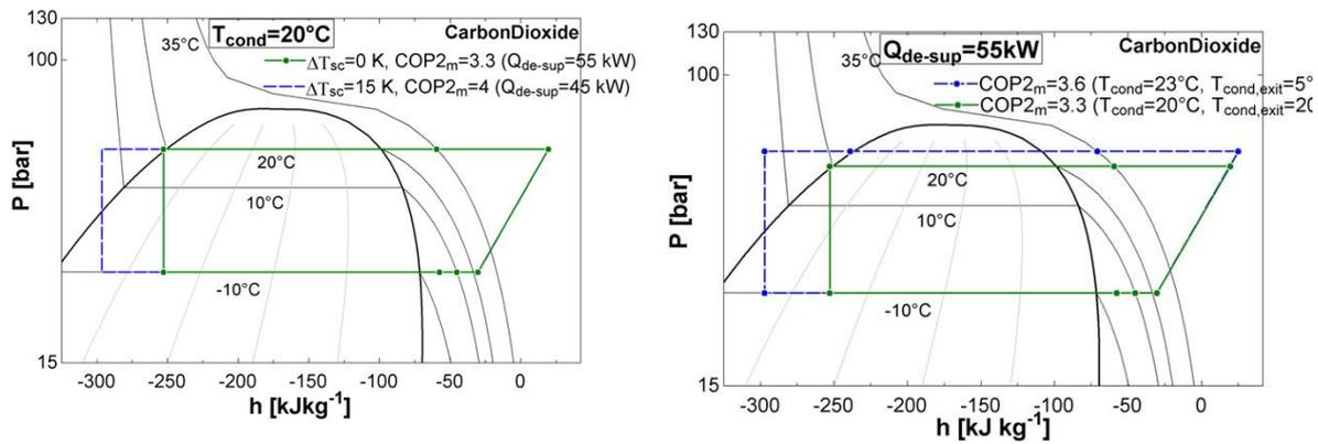
Figure 9 The impact of subcooling on a CO<sub>2</sub> system with heat recovery (Sawalha).
